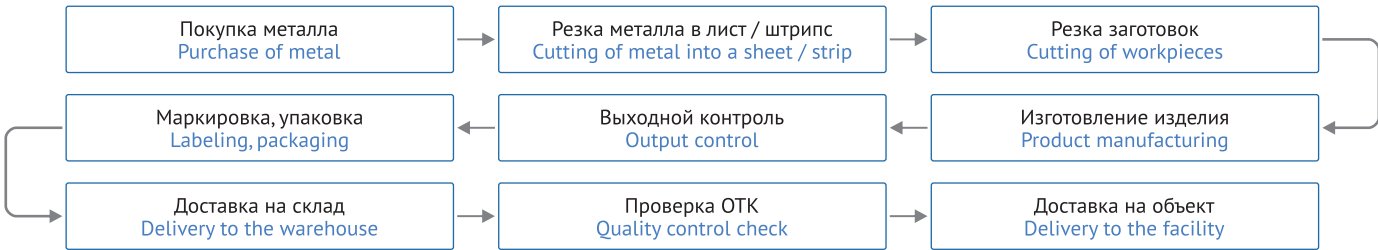
Рис. 4. Процесс изготовления изделий НФС Fig. 4. The process of manufacturing products of the hinged facade system
